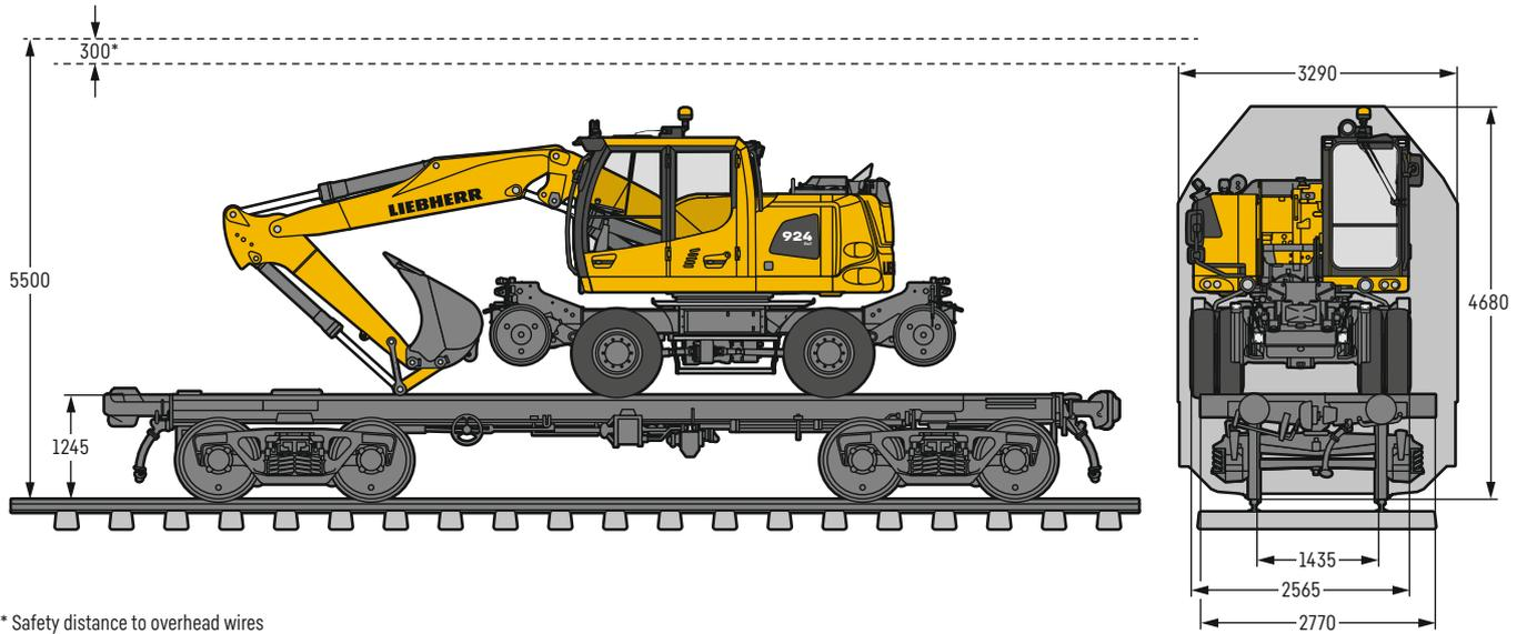
\* Safety distance to overhead wires
