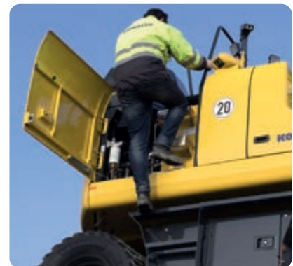
Handrails and anti-slip plates
