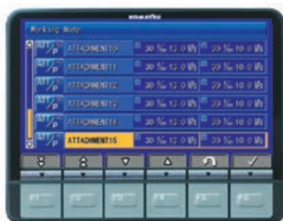
Komatsu Integrated Attachment Control (KIAC)
