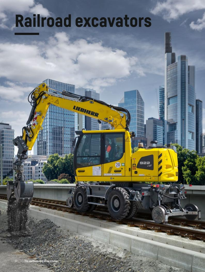
Liebherr has been developing rail-road excavators since 1967 and – as an OEM manufacturer – is the world market leader in this field. These machines are adapted to country-specific specifications (e.g. track width) and therefore comply with local conditions and safety regulations. Our rail excavators can be used either on the road or on railway tracks.
